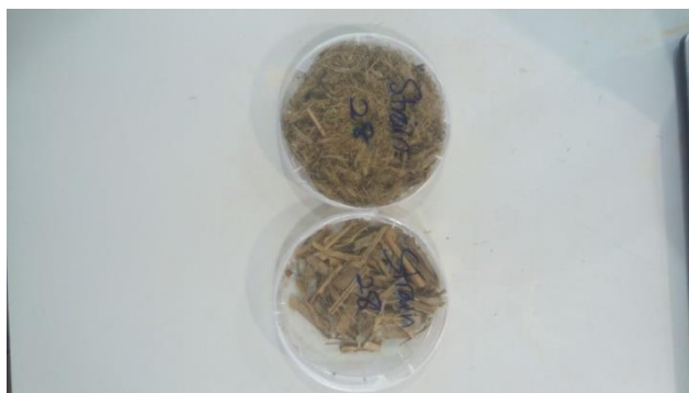
Figures of decomposed non-woody fiber. On the left is fermentative leaves and on the right is intact leaves that had been separated from fermentative leaves.
